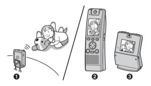
This feature allows you to monitor the room where the cordless camera ( $\bigcirc$ ) is located from the units ( $\bigcirc$ ,  $\bigcirc$ ). You can also monitor the room between the units ( $\bigcirc$ ,  $\bigcirc$ ).
